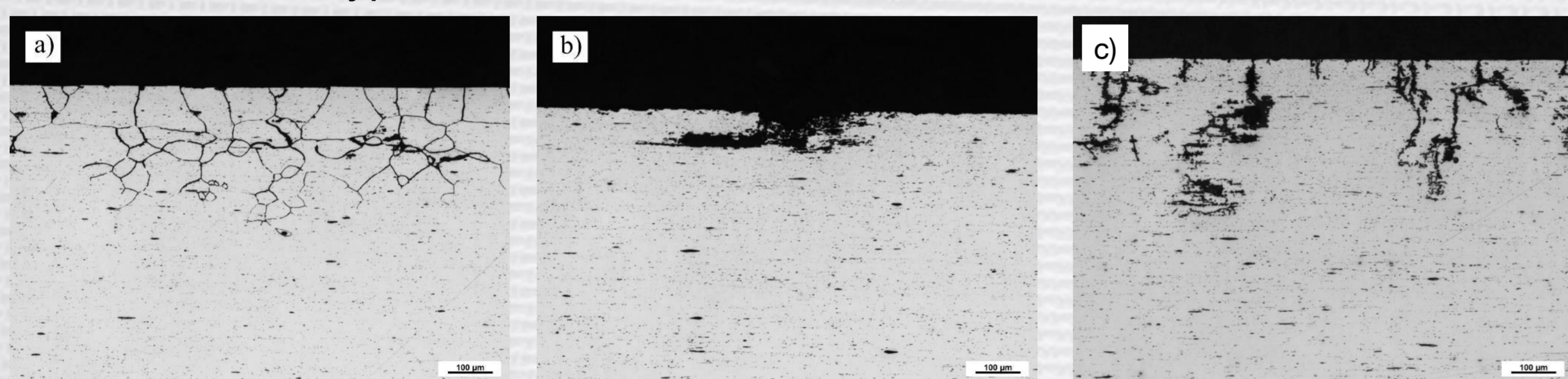
IGC - underaged condition from T1 and T2 temper
