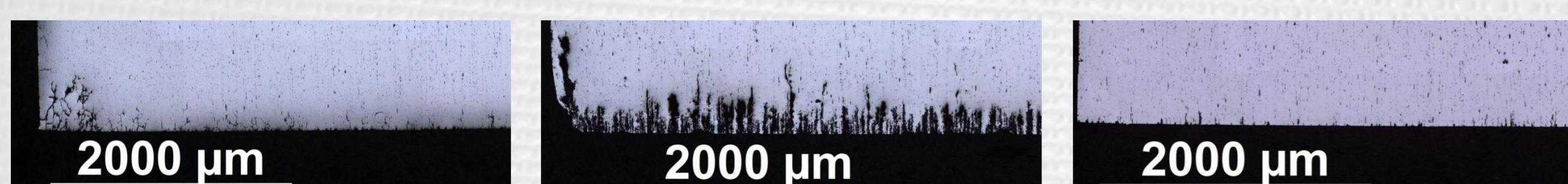
Temper T1 extruded + aging 160°C/4h+205°C/4h
