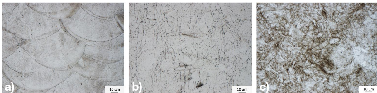
Figure 2. LM: a) as-built; b) solution annealing; c) precipitation hardening. Nital.
