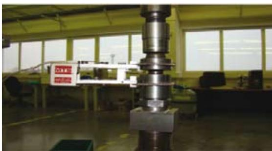
**Fig. 1. Detail of a test fixture for a SPT
