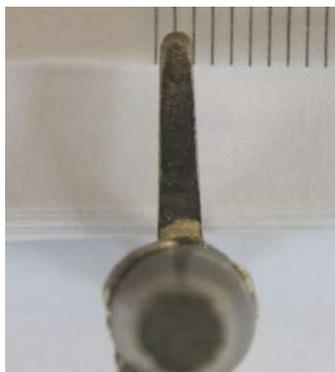
**Fig. 5 Conically tapered straight cavity**
