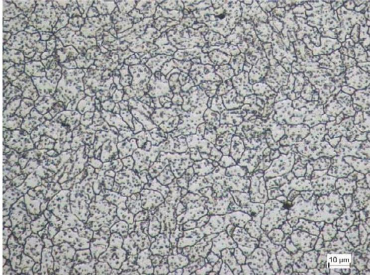
**Figure 1** Microstructure of a 1.2343 tool steel with visible prior austenite grain boundaries (G = 8)
