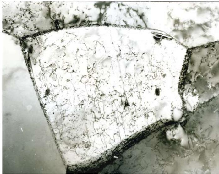
**Figure 7 Substructure of titanium Grade 1 in the initial state (X 10 000)**
