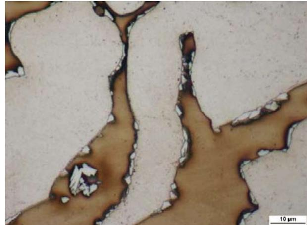
**Fig. 9. Sigma phase along grain boundaries, 1000x**
