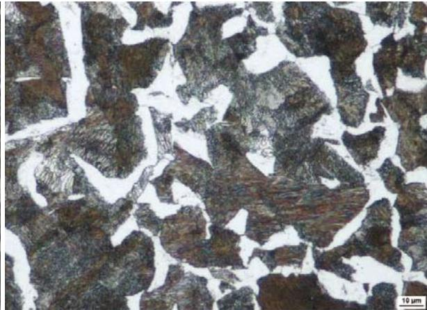
**Fig. 13 Microstructure of the AP at point P4, magnification 500, hardness 195 HV30**
