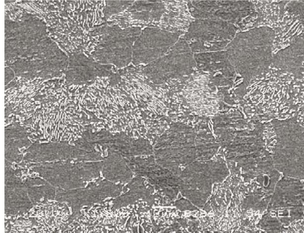
**Figure 4 The HT schedule: 710°C/12 hours, furnace cooling/30 hours. Partially spheroidized microstructure**
