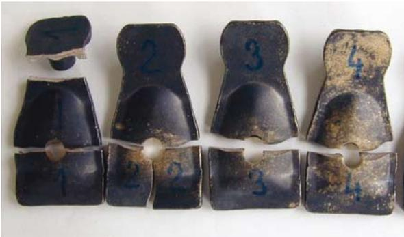
Figure 3 Damage of forgings occurring during punching holes and caused by the brittleness of material
