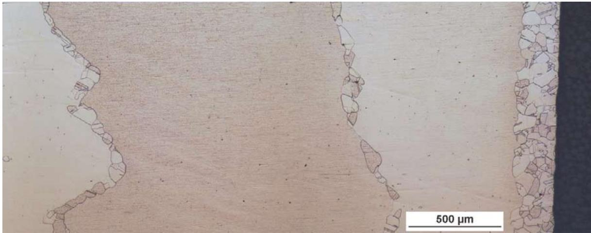
**Fig. 6 Preferential recrystallization of the Ni superalloy at grain boundaries and surface after cyclic hot forming.**
