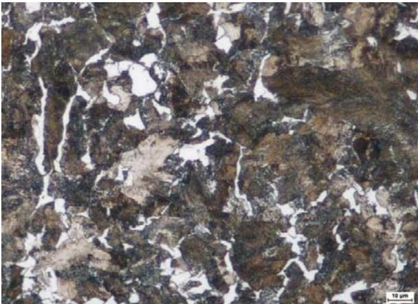
**Fig. 9** Microstructure of the AP at point P2, magnification 500, hardness 250 HV30
