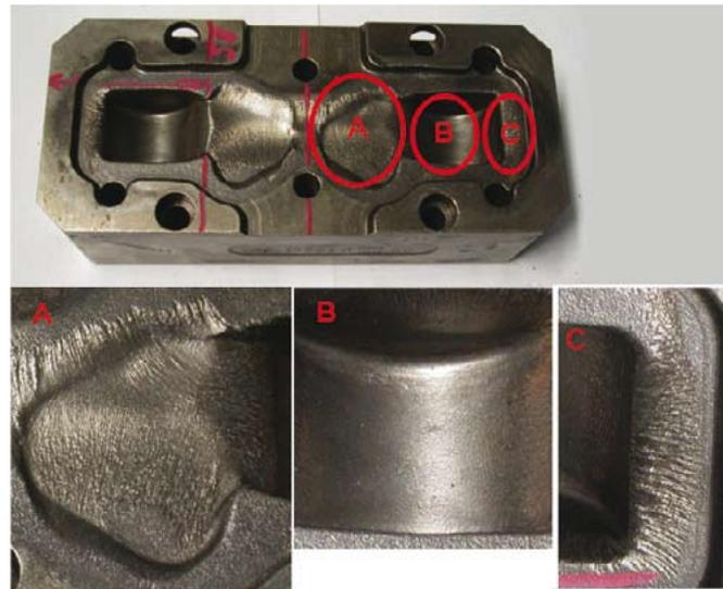
**Fig. 5 Forging die used for field tests and its worn surface**
