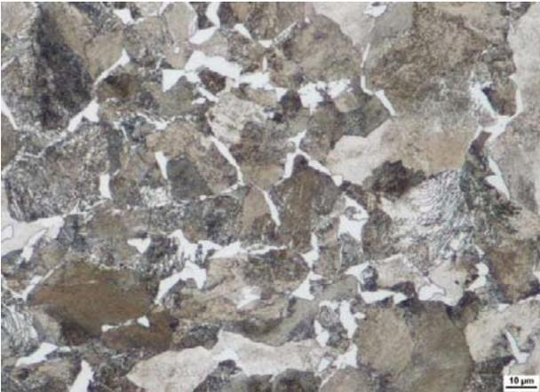
**Fig. 8** Microstructure of PS sample at point P1, magnification 500, hardness 234 HV30
