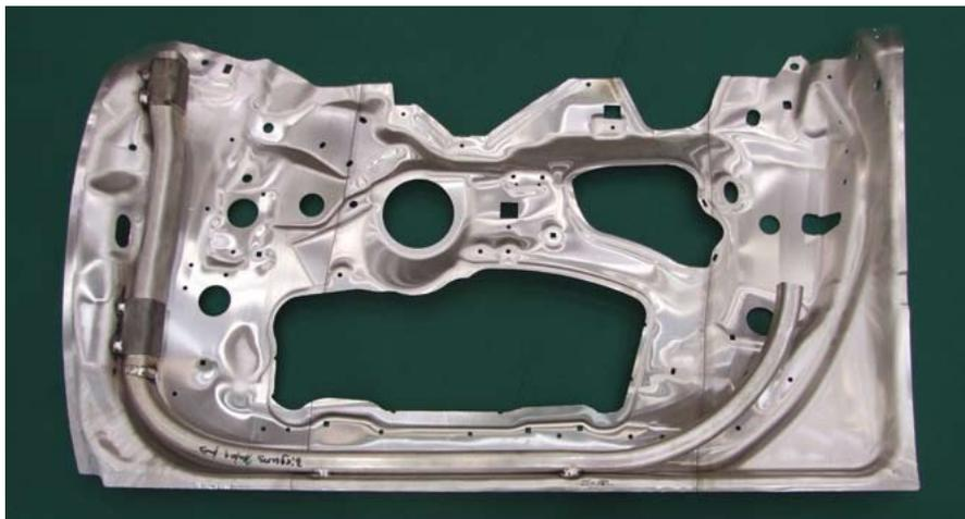
**Figure 1** The inside component of a passenger car door with a jointed frame made of a magnesium wrought alloy
