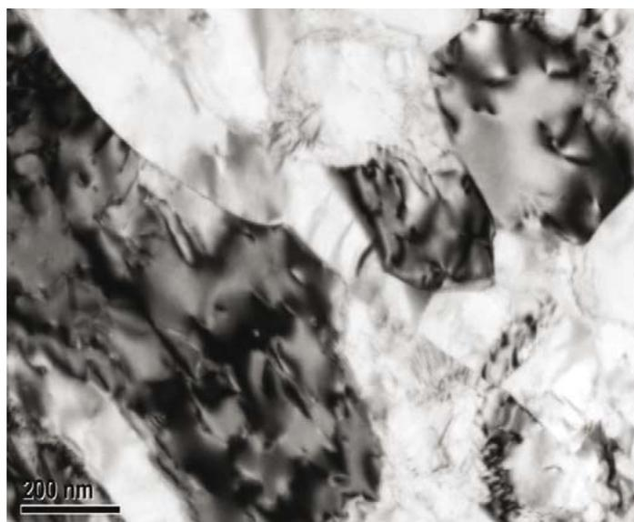
**Figure 8 Substructure of the sample after 8 ECAP passes**
