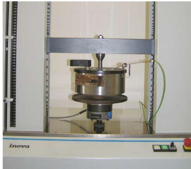
**Fig. 3 INOVA TSM 10 testing machine with testing apparatus for SP tests at reduced temperatures**
