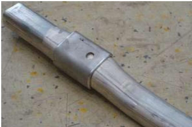
**Figure 2 Hydroformed jointed structural frame component with a hinge reinforcement (forming temperature = 300°C, forming pressure = 35 MPa)**
