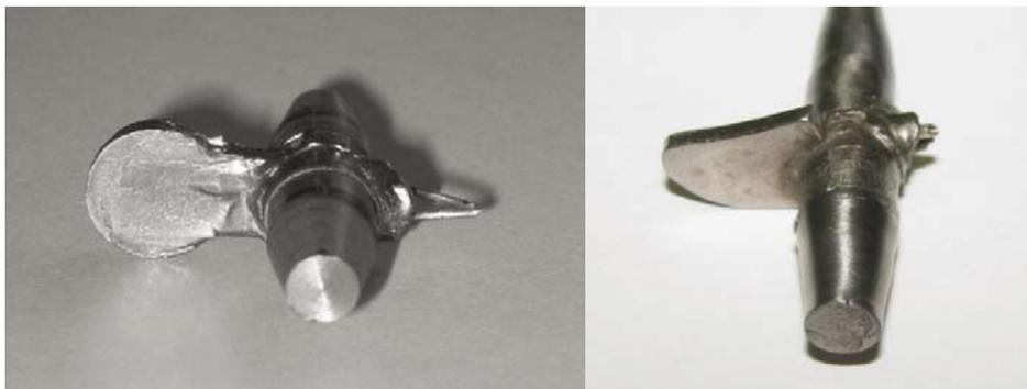
**Fig. 4 Completely filled cavities with tapered inlet opening**
